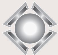
The system for carriage sliding is on hardened, ground, prism guides, which allows precise, straight cutting. Lasting precision is guaranteed by the exclusive assembly process. No glue is used to secure the guides, since the thickness could affect sliding. They are secured with a procedure for aluminium riveting along the entire length of the guide.
